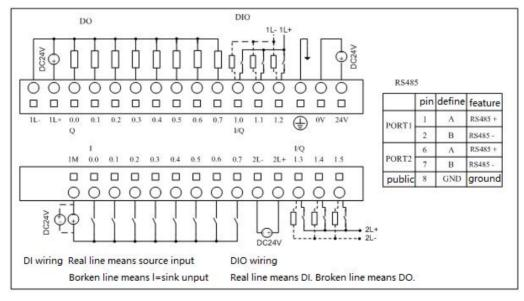
Fig.2-3 K205EX-22DT wiring diagram
