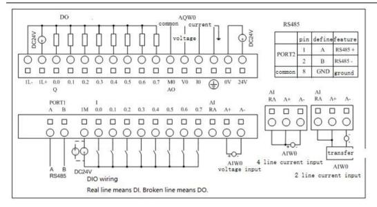
Fig.2-4 K205EA-18DT wiring diagram
