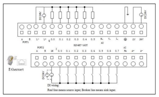
Fig.2-5 K204ET-16DT wiring diagram
