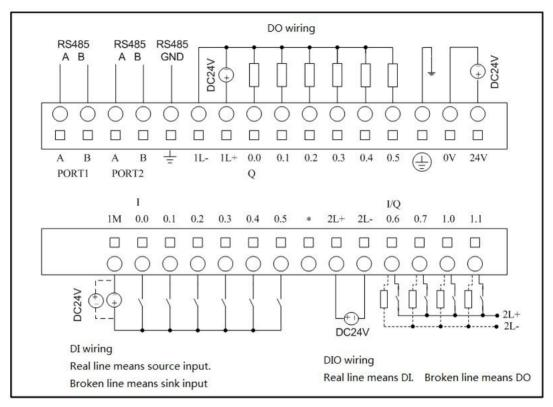
Fig.2-1 K205-16DT wiring diagram
